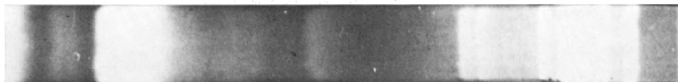
Fig. 18. Separation of flavines and derivatives. pH, 5.1; potential gradient, 100 V/cm; time, 90 min.
